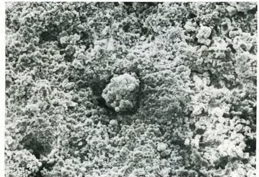
Fig. 25. Biological attack. Marble "pitting" by black yeasts. The yeasts have a shape similar to Pentelic marble crystals and penetrate deep, sometimes also by hyphae formation. Theatre of Dionysus. (Scanning electron micrograph, Krumbein).
