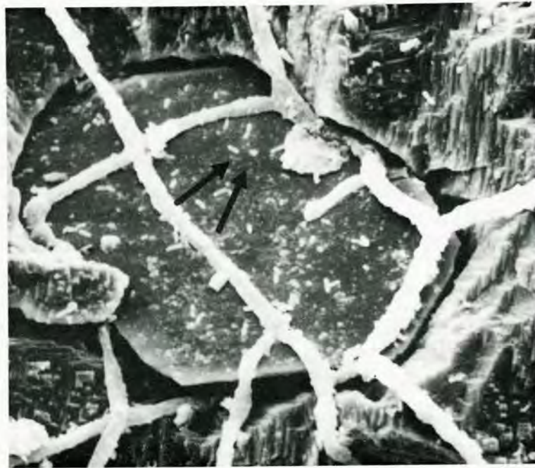
Fig. 24. Biological attack. Fungi penetrating under a marble grain and detaching it. Parthenon. (Scanning electron micrograph, Krumbein).
