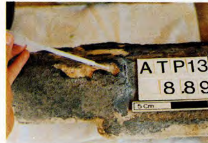
Fig. 42. Impregnating disintegrated marble to restore the coherence of the crystals.
