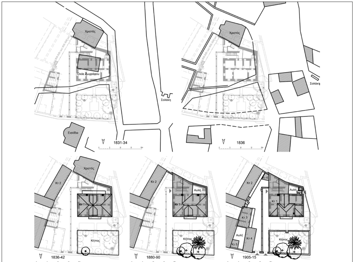
The main building phases of the listed building at 13, Polygnotou Street. Study-Drawing: K. Skaris, 2020
