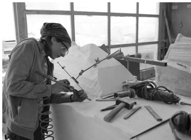
The traditional method of creating new marble additions with the use of a pointing device. Photos K. Skaris, 2020
