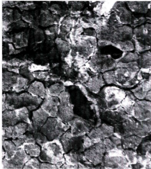
Fig.3, Sulfated grain boundaries, after their washing with water and consequently the removal of gypsum. The grains are ready to be detached.
