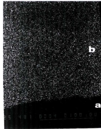
ii. EPMA X-rays x 400. a Marble, b gypsum. Identification for S
