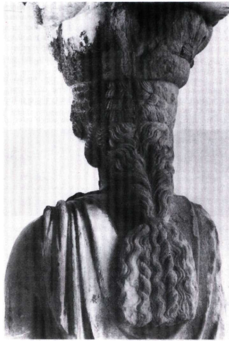
Fig.5. Sulfation on the back of a Caryatid. Rear surface protected from rain water. The details are preserved.
