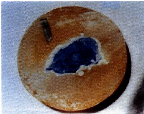
Fig. 26a, b, c, d. Areas of \text{Ca(OH)}_2 (blue-gray) and of calcium carbonate. a: Carbonation in the presence of 25% \text{CO}_2 , b: Carbonation in the presence of 25% \text{CO}_2 and 6% \text{CaCO}_3 in the \text{Ca(OH)}_2 c: Carbonation in the air without 6% \text{CaCO}_3 , d: Carbonation in the air with 6% \text{CaCO}_3 .
