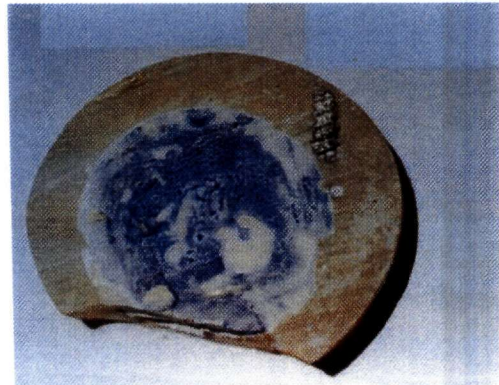
Fig. 26a, b, c, d. Areas of \text{Ca(OH)}_2 (blue-gray) and of calcium carbonate. a: Carbonation in the presence of 25% \text{CO}_2 , b: Carbonation in the presence of 25% \text{CO}_2 and 6% \text{CaCO}_3 in the \text{Ca(OH)}_2 c: Carbonation in the air without 6% \text{CaCO}_3 , d: Carbonation in the air with 6% \text{CaCO}_3 .
